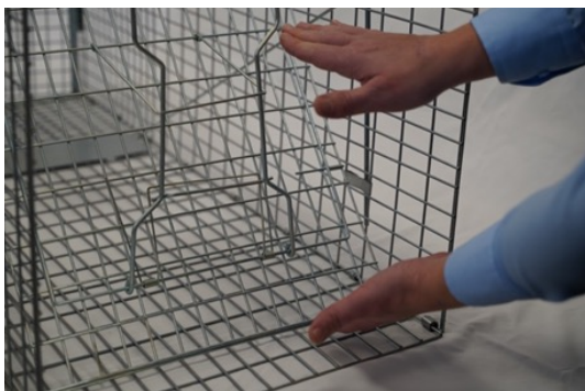
10: Open the front of the cage by pushing the top part of spring on the trap door and lift the door upwards from the bottom
