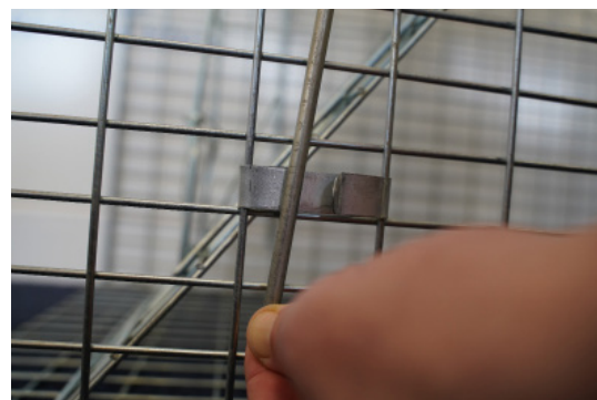
4: On top of the cage is a u shape bar that clips into both sides of the cage in order to keep the cage rigid
